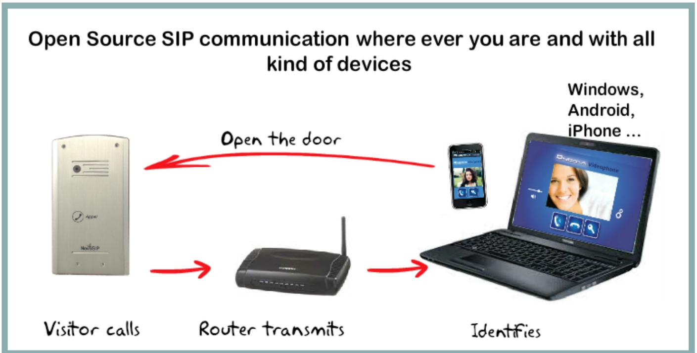
The door station NovoSIP includes a great internal SIP server FreeSwitch for residential or office: no need to have an external SIP server in your installation. Just connect the NovoSIP to your router or switch and enter the local IP address in the device you want to communicate. You can also use an external SIP server your choice.
